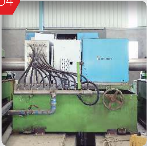
Inline Annealing (Heat Treatment)
